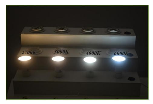
It is a poor metric for LED lighting because an LED spectrum is unlike that of a glowing filament. For example, a 4000K filament would have a peak output at a wavelength of about 725 nm, but that of an LED could be around 450 nm.
